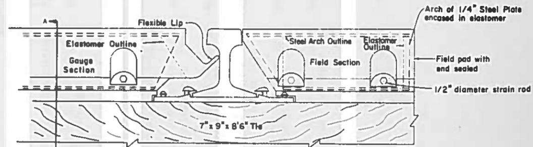
Arch of 1/4" steel plate encased in elastomer. Each 18" pad spans one (1) 18" tie space center to center. No shims required - Pads manufactured to fit rail height.
