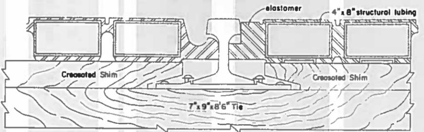
4"x8" structural steel tubing (0.188" wall thickness) encased in elastomer. Each 80" pad spans four (4) 20" tie spacings center to center.
